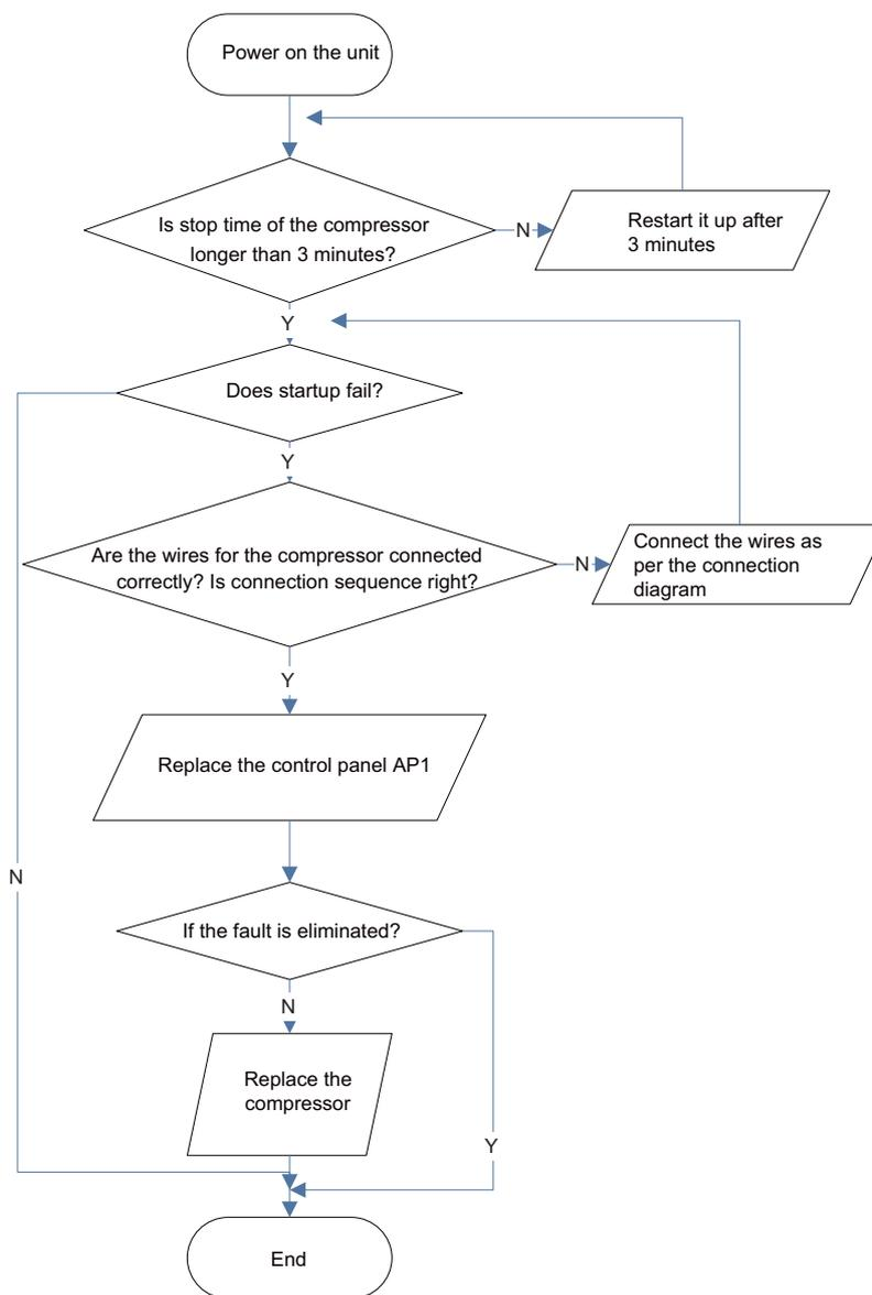
**(6) Overload and air exhaust malfunction diagnosis (following AP1 for outdoor unit control board)**
