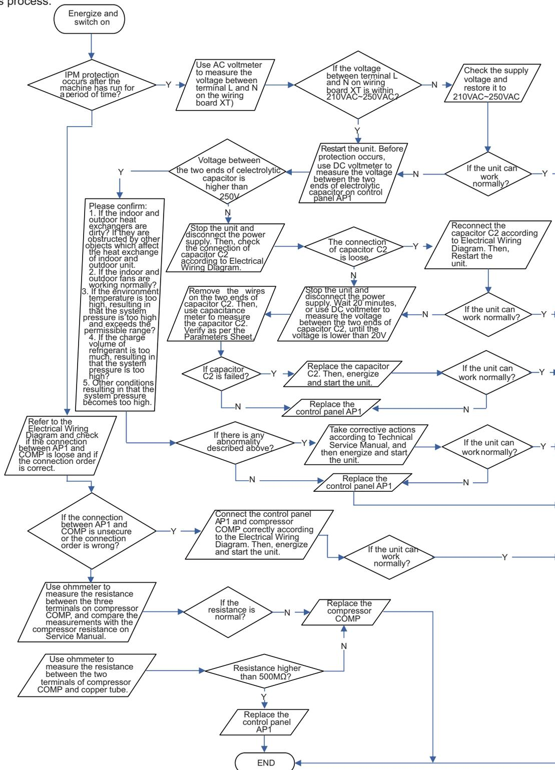
**(4) Start-up failure (following AP1 for outdoor unit control board)**
